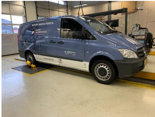
Figure 4 Test car on the chassis dynamometer and the WLTP test cycle used for transient testing.
